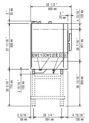
CWII Cold Water inlet 1 CWI2 Cold Water Inlet 2
